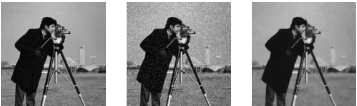
Figure 3.4: Image denoising model problem ( Example 3.3 .) Left: original image (dimensions n_1 = n_2 = 256 ). Middle: image with noise. Right: denoising result obtained using 200 iterations of the Chambolle-Pock Algorithm 3.6 with \sigma = 1 and \tau = 1/10 and weighting parameter \beta = 0.08 .
